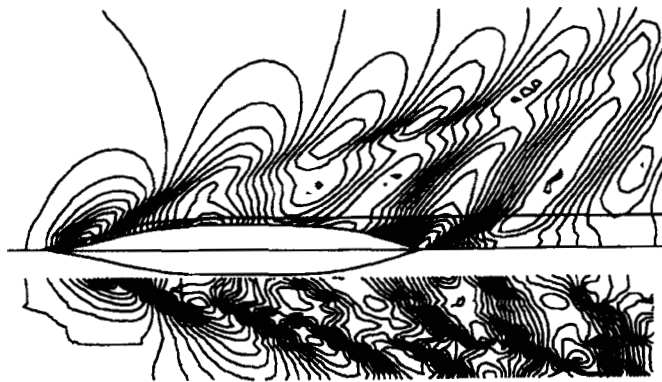
Figure 19. Free surface elevation: comparison between numerical results (top half) and experimental data 26 (bottom half) for the S60— Fr = 0.300 . Levels of \mathcal{H}/Fr^2 : -0.1, -0.09, \dots, 0.1
